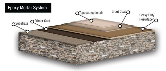
Epoxy Mortar Flooring System is a troweled, high strength concrete resurfacing material. It is used for environments requiring an industrial grade floor or when a concrete floor has sustained damage requiring a 3/16" to 1/4" surface restoration.
